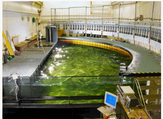
Figure 13: University of Edinburgh Curved Wave Tank (source: Edinburgh Wave Power Group)
