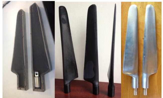
Figure 3 Photographs of blades: (left) composite blades during manufacturing [19]; (middle) composite blades; and (right) aluminum blades.
