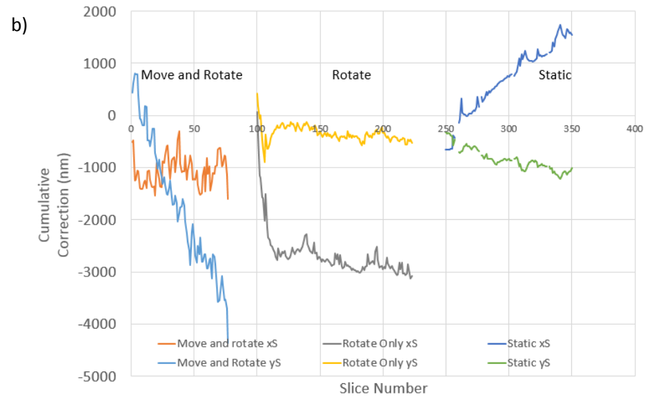
Figure 6. SEM beam displacement (drift correction) a) change from slice to slice and b) cumulative change from start of milling
