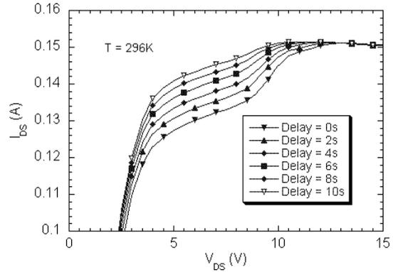
Fig.4. Relaxation of the collapsed region at 296K.
