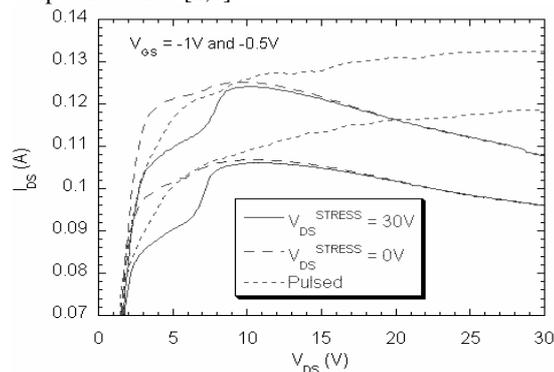
Fig.1.  $I_{DS}(V_{DS})$  at 296K for various measurement conditions.
