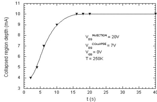
Fig.3. Evolution of the collapsed region depth after a  $V_{DS}=20V$  stimulus applied during  $t$  seconds, at  $T = 250K$ .
