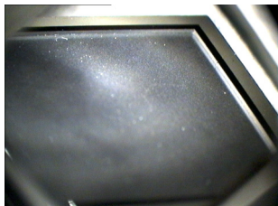
(a): Etched Si cover with SnPb
