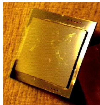
(c): Demonstrator after brazing of the cover
