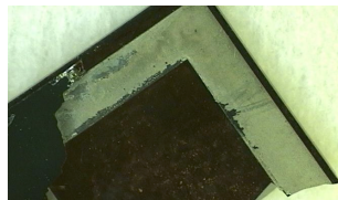
(b): Brazed cover after shear test
