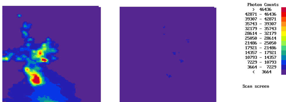
Figure 3.6: The effect of repeat IR scanning on signal levels obtained from a mixed feldspar sample containing 99% unirradiated grains and 1% irradiated grains.
