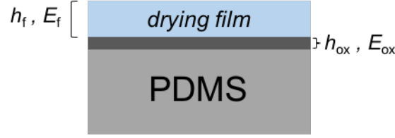
FIGURE 7.7: Schematic of the trilayer structure resulting from solution deposition (and planar film formation) on oxidised PDMS.
