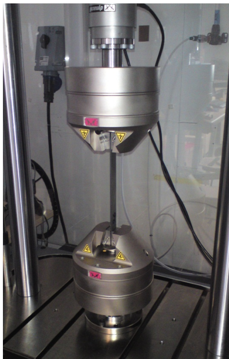
Figure 7 - Testing of the specimen using an Instron E10000 tension-torsion machine.
