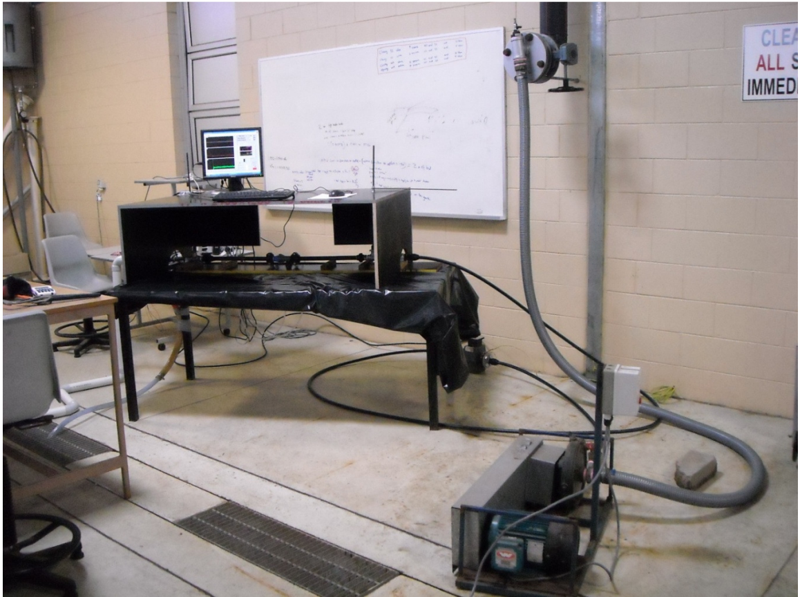
Figure 3.5 – Stage two testrig Automatic data acquisition with higher input heads
