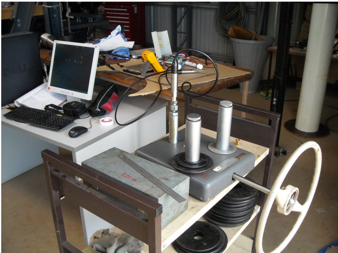
Figure 3.1 – Dead weight pressure tested calibrating the pressure transducers
