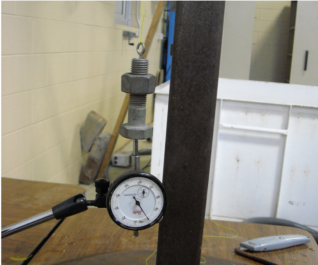
Figure 3.7 - Dial gauge overview used for tubes movement
