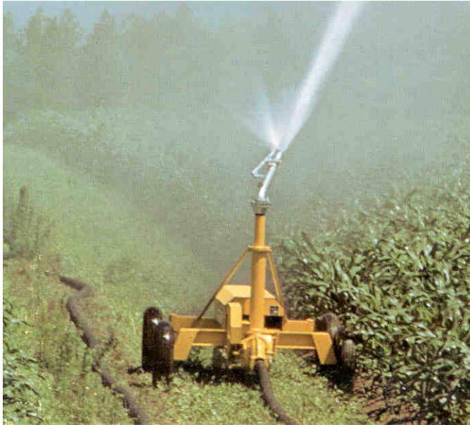
Figure 1.3 – Cable tow travelling gun irrigator fed by flexible soft hose
