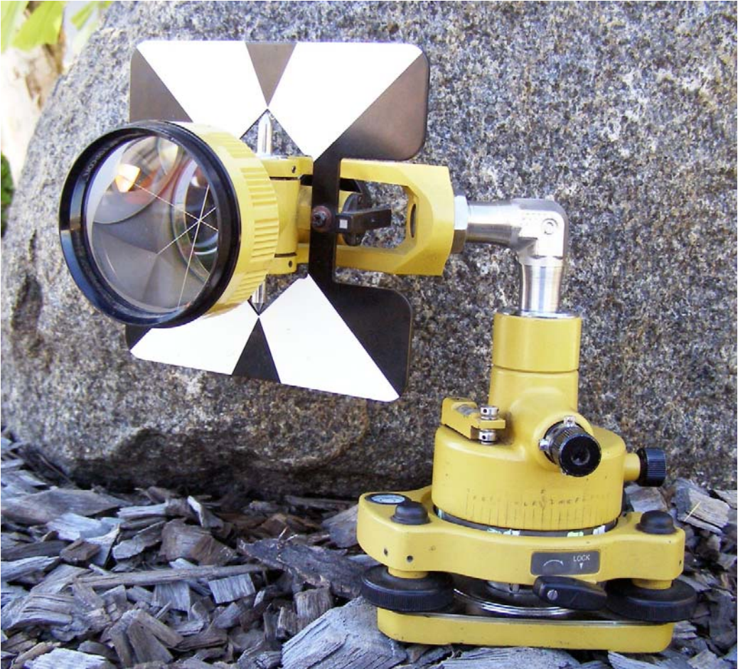
Figure 3.10: Standard round prism on 90 degree prism adaptor.
