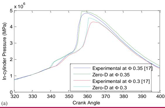
Figure 3 Effect of equivalence ratio on the incylinder pressure: CR=10.0, N=900 rpm, T<sub>in</sub>=40°C, P<sub>in</sub>=95 kPa (a) Validated varying equivalence ratio.
