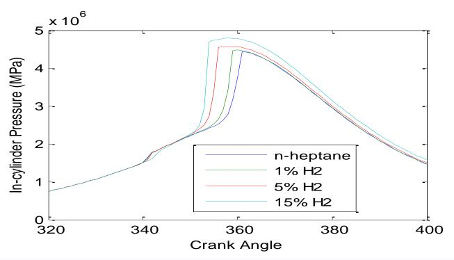
Figure 4 Predicted effect of hydrogen addition on the incylinder pressure for fixed n-heptane injection: CR=10.0, N=900 rpm, T<sub>in</sub>=40°C, P<sub>in</sub>=95 kPa
