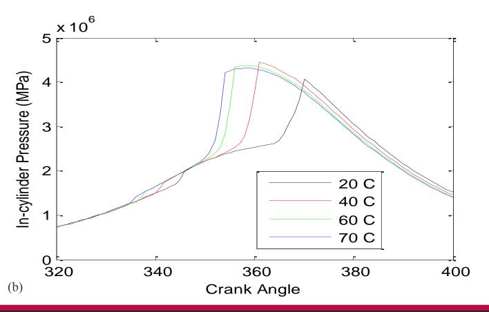
Figure 2 Effect of intake temperature on the in-cylinder pressure: CR=10.0, N=900 rpm, P<sub>in</sub>=95 kPa, AFR=50 (b) Predicted incylinder pressure trend.
