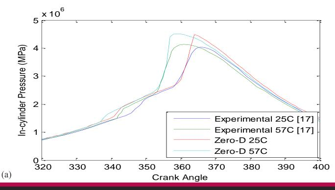
Figure 2 Effect of intake temperature on the in-cylinder pressure: CR=10.0, N=900 rpm, P<sub>in</sub>=95 kPa, AFR=50 (a) Validated varying intake temperature.
