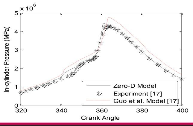
Figure 1 Comparison between single-zone zero-dimensional model with experiment and another single-zone model using modified Woschni heat transfer model [17]. CR=10.0, N=900 rpm, T<sub>in</sub>=40°C, P<sub>in</sub>=95 kPa, AFR=50.
