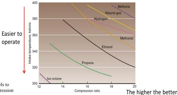
**Figure** Intake temperatures required for fuels to operate under HCCI mode with various compression ratios (Aceves & Flowers 2004).
