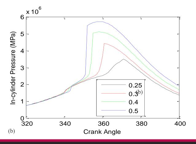
Figure 3 Effect of equivalence ratio on the incylinder pressure:
