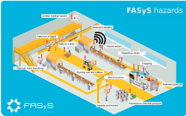
Figure 2. FASyS 13 prevalent hazards
