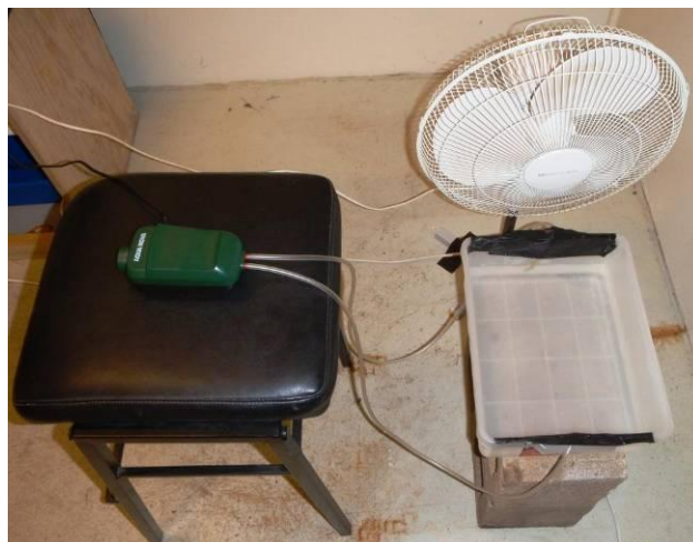
Figure 2: An example experimental setup with the fan positioned close to the surface of the small water tank and the water aeration/bubbler system, with its two air outlets attached at opposite ends of the small tank wall.
