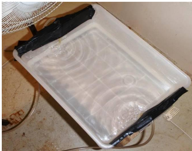
Figure 4: Outlet bubblers from the water bubbler in operation. The even outwards circular spread of the capillary waves can be clearly seen.
