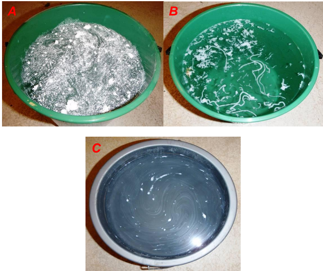
Figure 1: A) WaterSavr chemical film unevenly spread out over a water surface. B) Aquatain chemical film randomly distributed over a water surface. C) Octadecanol monolayer spread on top of a water surface.
