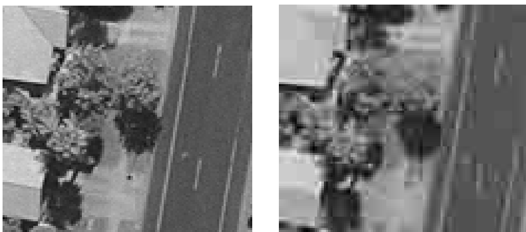
Figure 5: A JPEG version (right, section only) of the aerial view ( 1000^2 ) for a compression ratio of 10:1 and the same image reconstructed using the vertices of contour lines with increments equal to 8 (left, same section).
