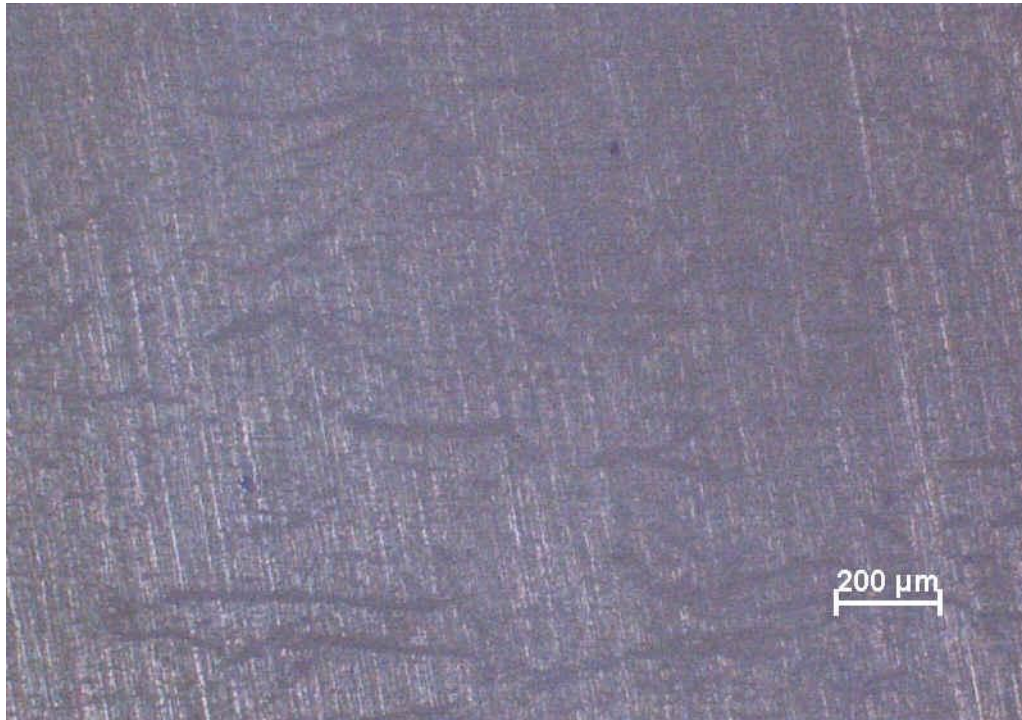
Figure 6. Micro graphs of cut-off view (along the longitudinal direction of the sample) of the silk fibre/PLA composite with 5 vol% silk fibre
