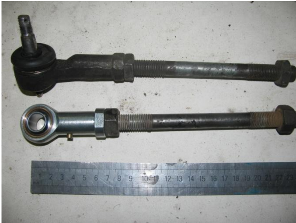
Fig. 4.2.1.3 Tie Rod End - Length difference
