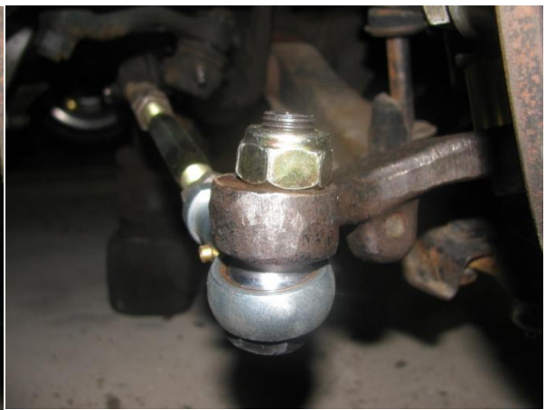
Fig. 4.2.1.8 Tie Rod free from binding
