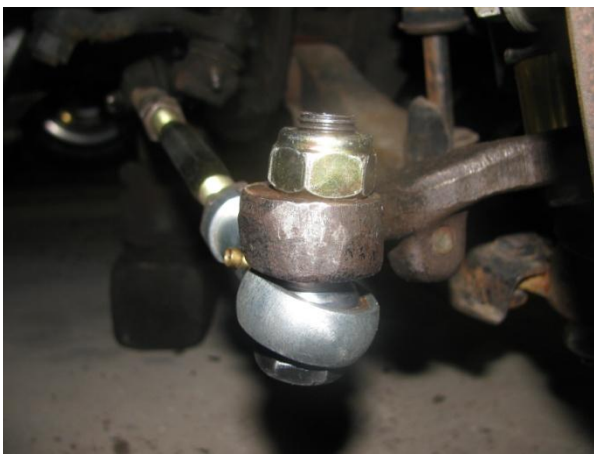
Fig 4.2.1.7 Tie Rod free from binding
