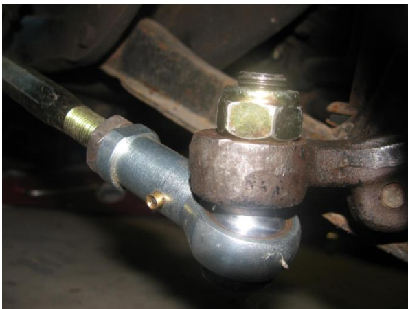
Fig. 4.2.1.9 Tie Rod free from binding
