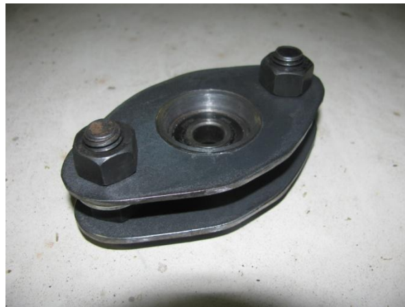
Fig. 5.1.4 Pivot before Welding
