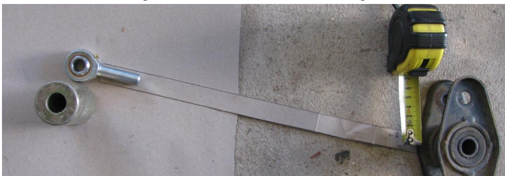
Fig. 5.1.3 Watts Link Travel – Differential 70 mm Higher
