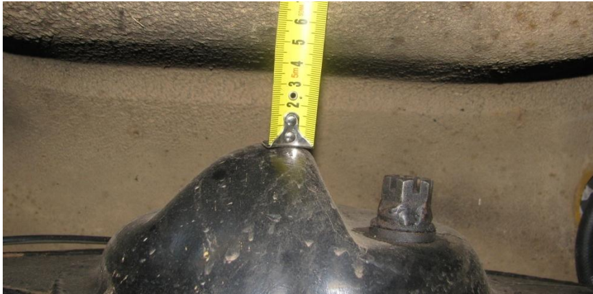
Fig. 5.1.1 Standard Clearance for Watts Link
