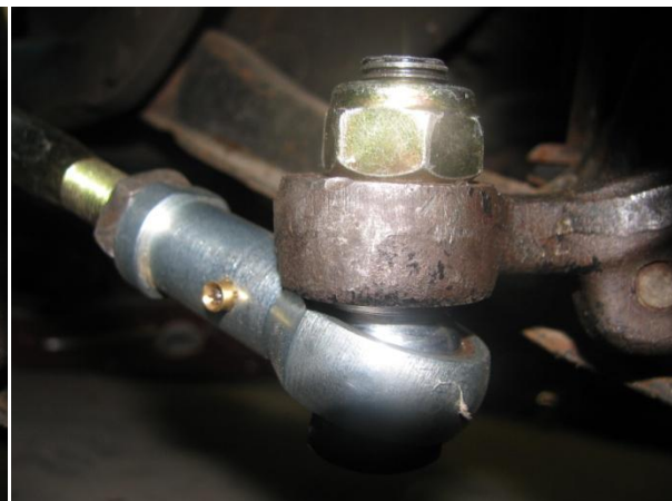
Fig 4.2.1.10 Tie Rod free from binding
