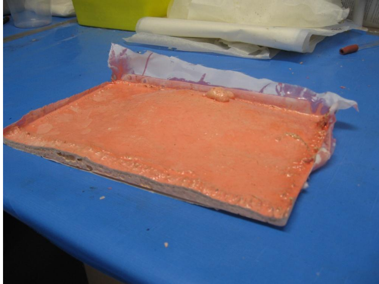
Figure 9 – Sample with excessive resin without compression during curing
