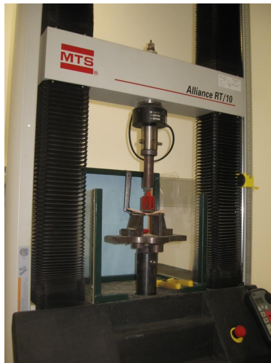
Figure 12 - Flexural 3 point test
