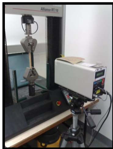
Figure 11 – Tensile testing with laser extensometer in place.
