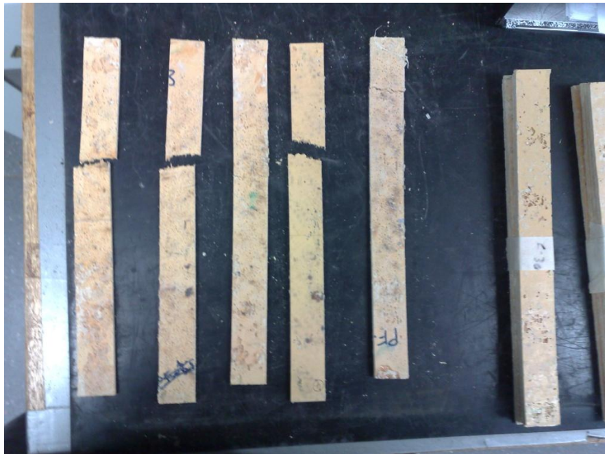
Figure 16 - Tensile testing failure
