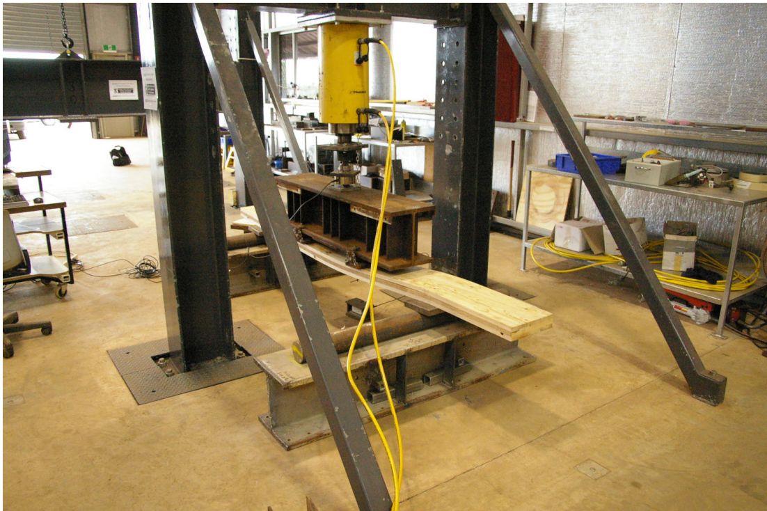
Figure 5.8: Four Point Bending Test: Post Failure
