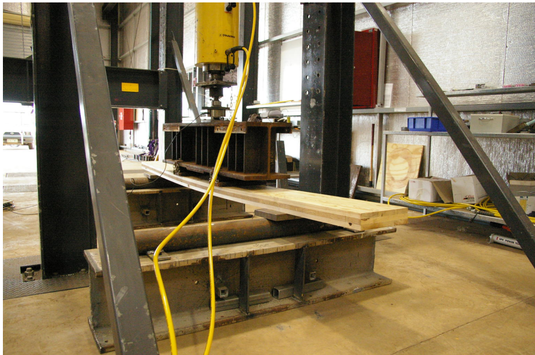
Figure 5.7: Four Point Bending Test:Elastic Region
