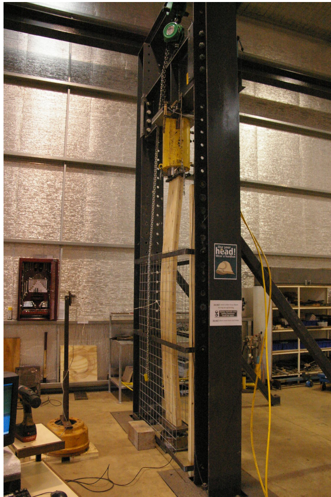
Figure 5.1: Sample 1, Post Ultimate Load Deflection
