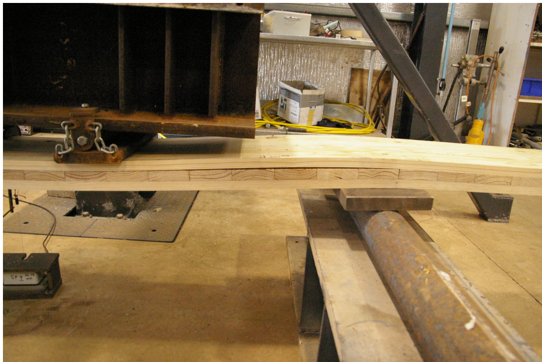
Figure 5.9: Delamination of CLT Due To Flexural Shear
