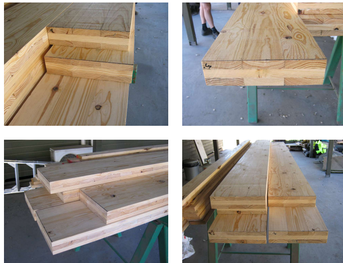
Figure 4.4: CLT Samples Fabricated by Hyne
