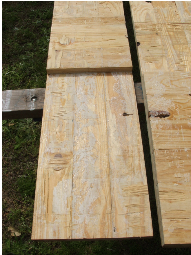
Figure 5.6: Sample Three Delaminated Glue Surface
