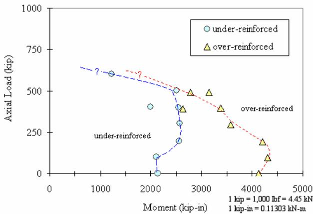
Figure 4. Strength interaction diagram of concrete-filled FRP tube [36].
