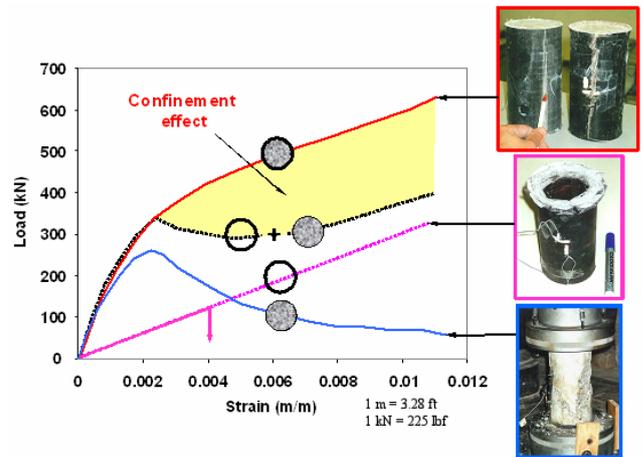
Figure 3. Confinement effect of FRP shell on concrete [19]
