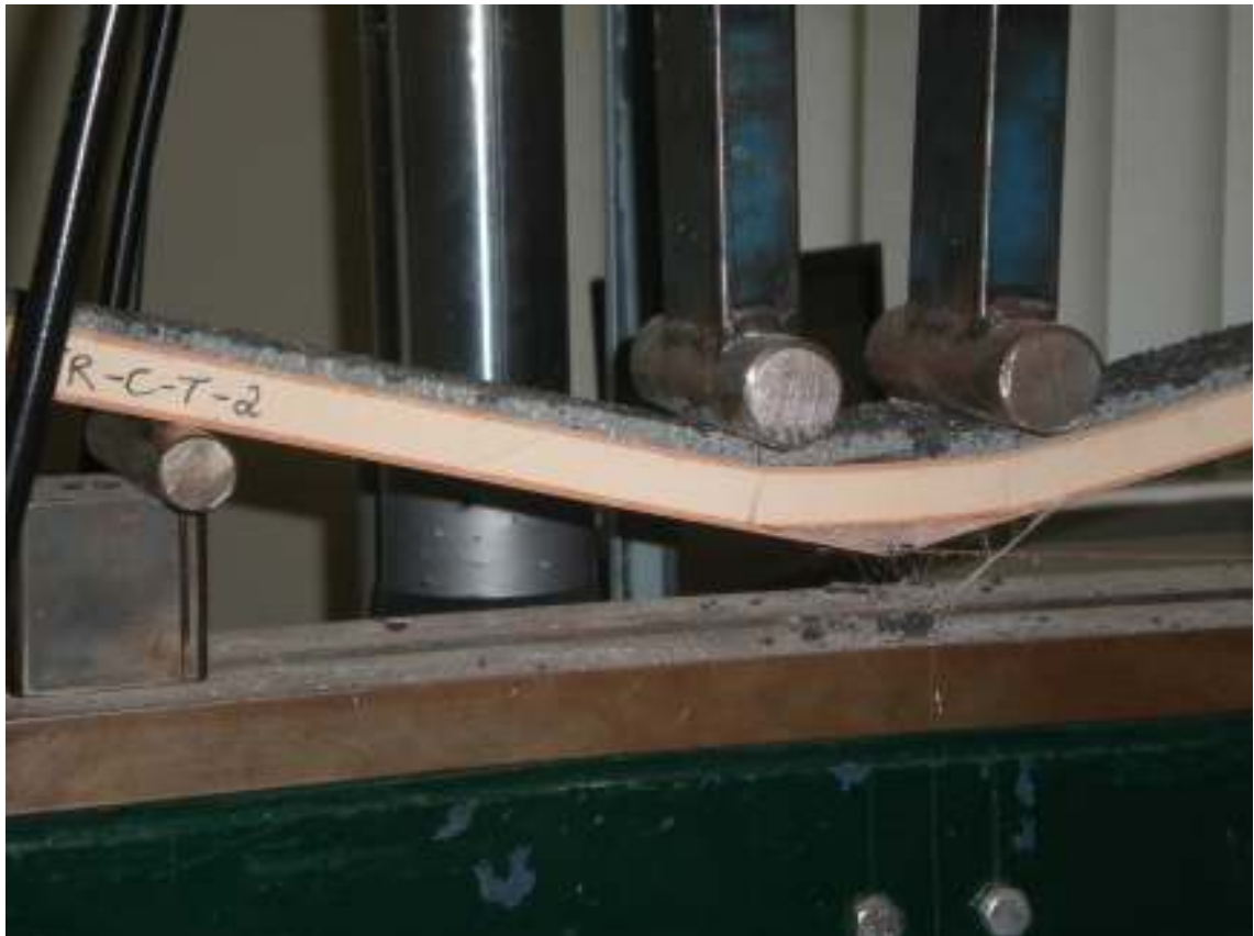
Figure 4.16 Sandwich Panel With Cover Cut damage
