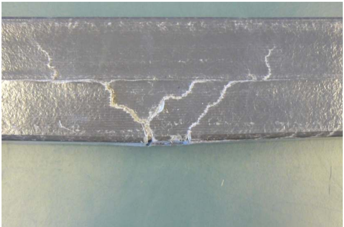
Figure 6.16 Cut Failure in 50x50mm section
