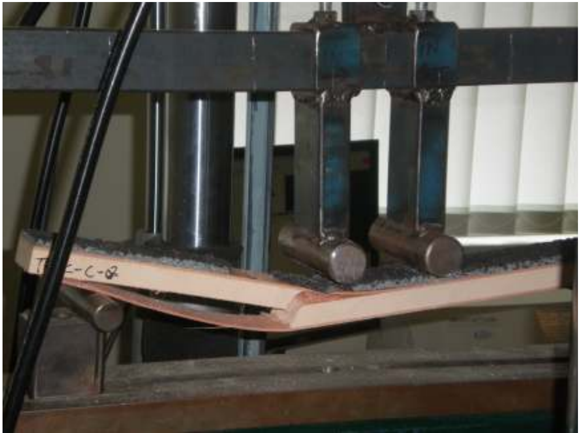
Figure 4.8 Failure of Sandwich Panel with Cover
