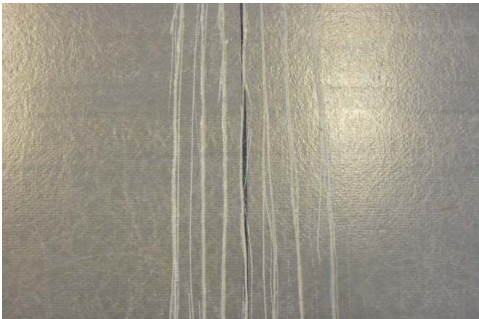
Figure 6.6 Cut Damage to Exel Composite
