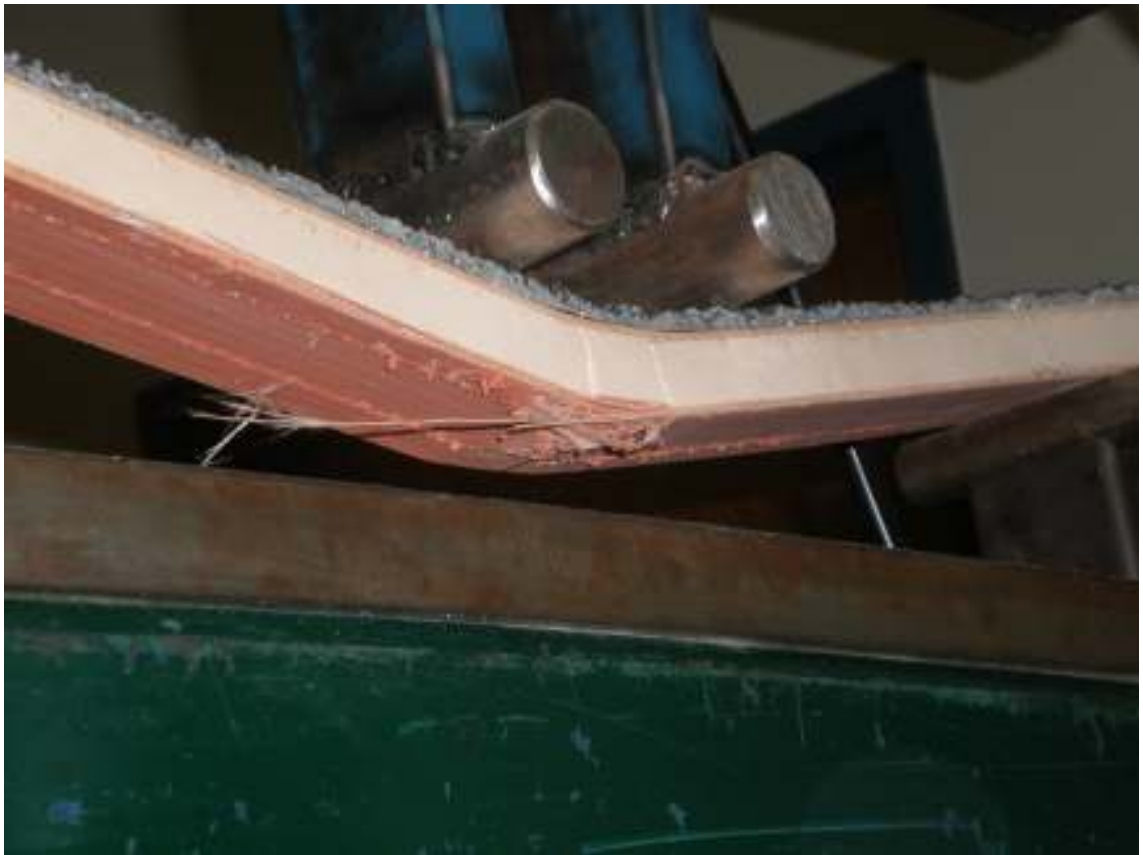
Figure 4.13 Failure of Sandwich Composite with Cover Sharp Impact Damage
