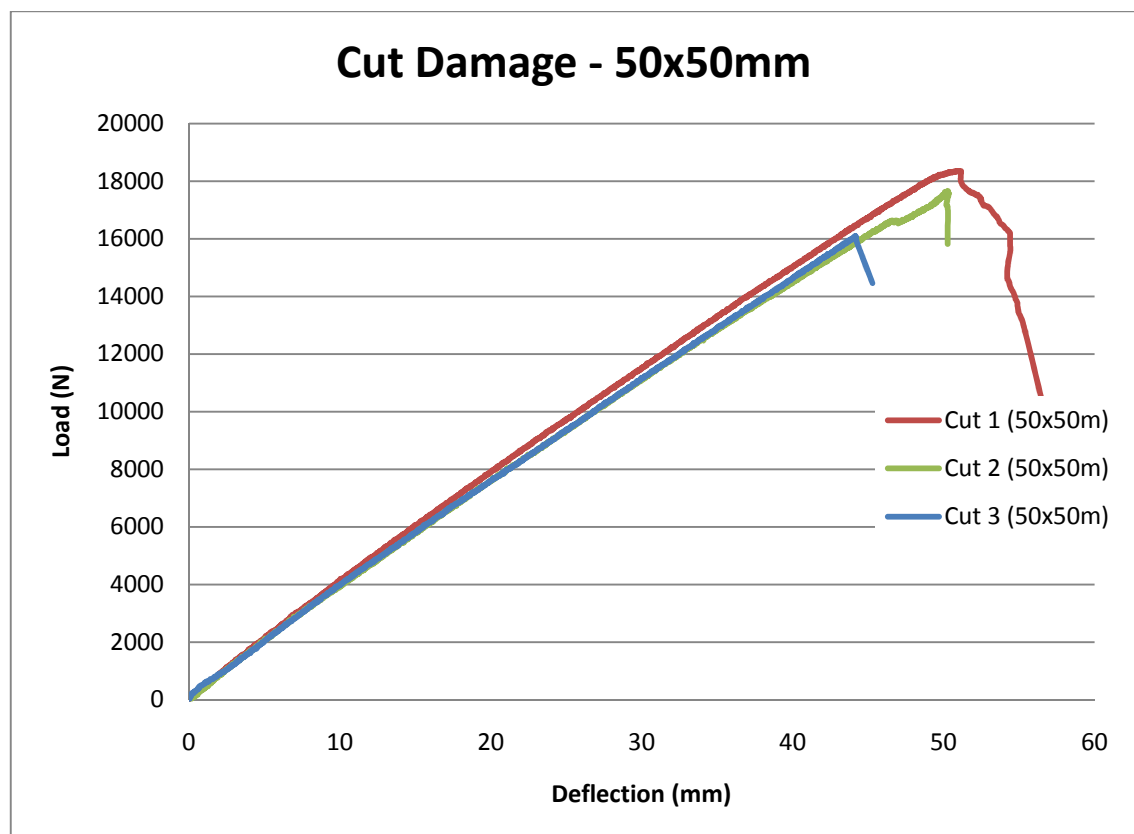
Figure 6.17 Cut Damage Results of 50x50mm Samples
