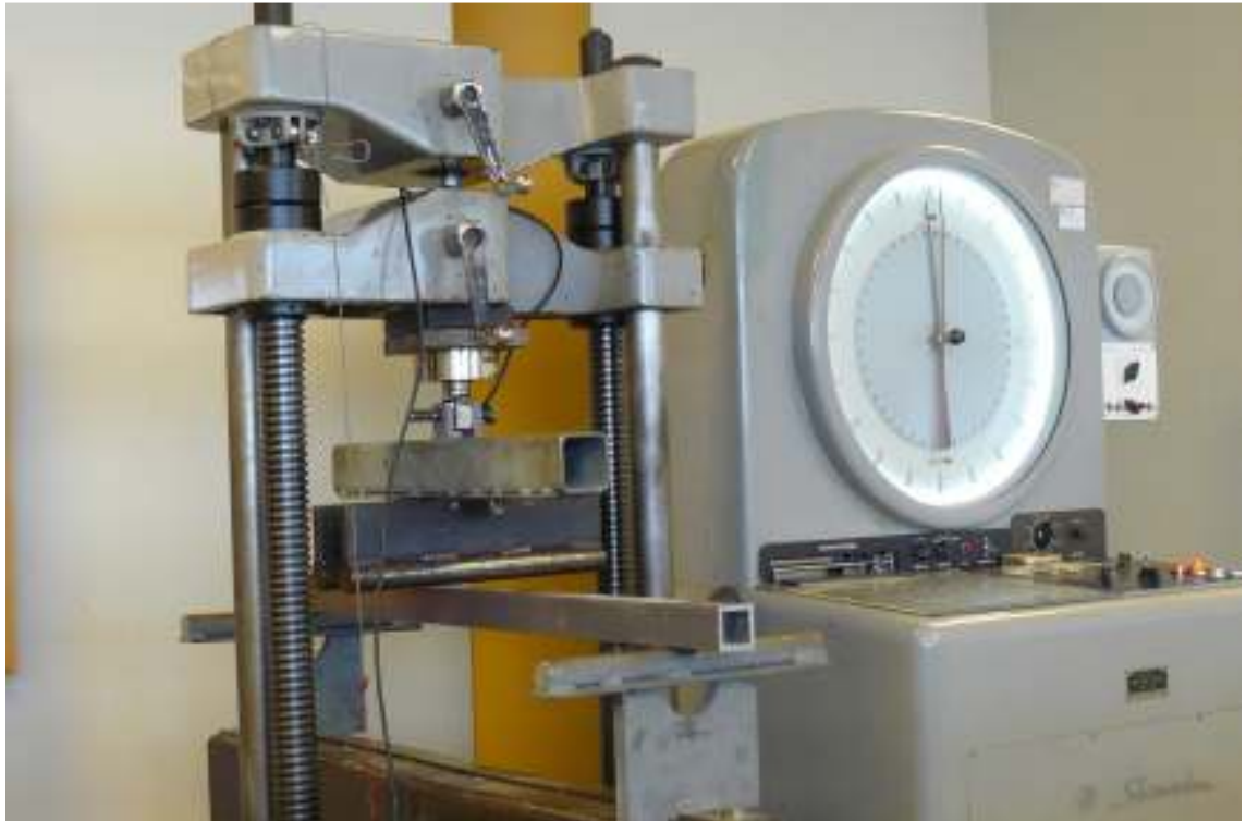
Figure 3.12 MTS testing machine used on the Pultrusions
