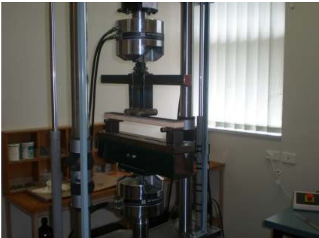
Figure 3.11 MTS testing machine used on the Sandwich Panels
