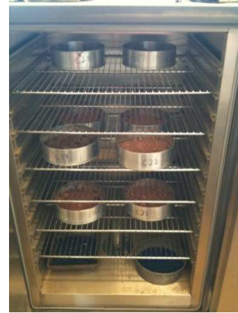
(18) Figure 3.3.4.3 – Specimens placed in oven
