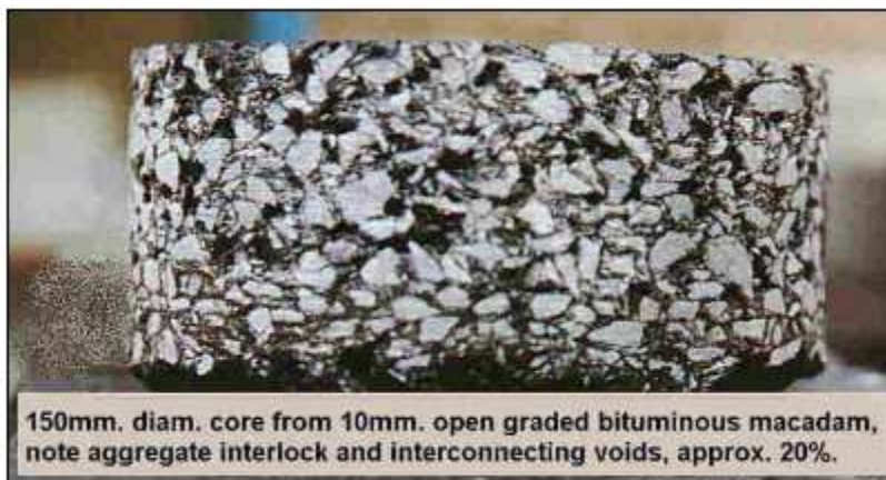
(6) Figure 2.3.1 – Core sample of open graded asphalt
