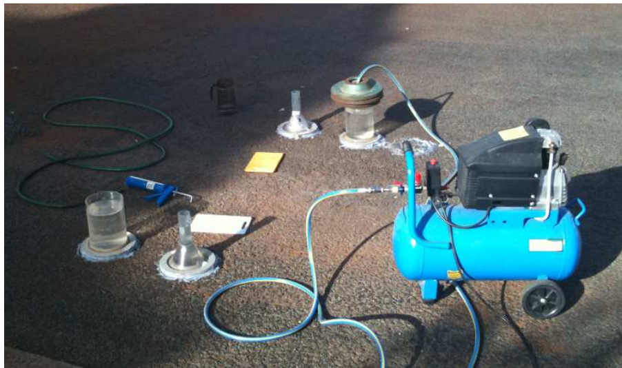
(27) Figure 3.5.4.2 – Pressurised testing in process
