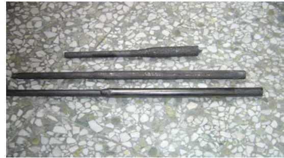
Fig. 4: Assemblies being taken from various passes of the drawing operation
