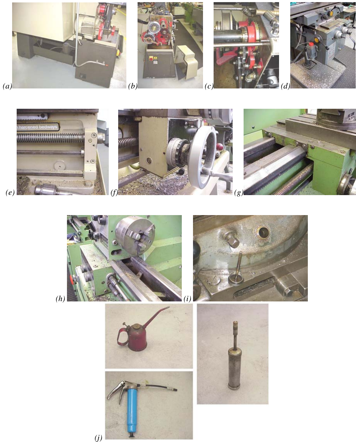
Figure 2 Some of the parts and features covered by the maintenance related tours of the workshop. Concepts explained: (a) inspection of belts, (b) need to switch off machines before covers are taken off, (c) safety interlocks need to be inspected and filling/emptying points in the headstock were shown, (d) some machines included hand-operated pumps to deliver lubricating oil to selected machine parts, (e) lubrication of lead screw supports and the feed rod, (f) monitoring point for apron (gearbox) oil level and the hand pump used to lubricate the carriage slideways, (g) inspection of slideways and wear on chip guards, (h) monitoring point for headstock (gearbox) oil level and points where the oil for the feedbox could be replenished and drained, (i) an oil level dipstick and filling point on a milling machine knee and (j) tools used for lubricating the machine tools investigated.
