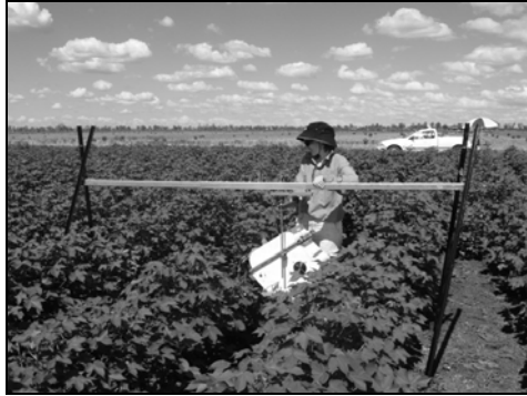
Figure 2. Manually moved camera enclosure in a cotton crop.
