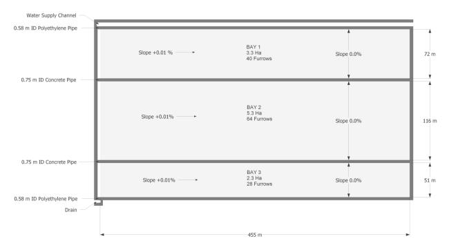
**Figure 2:** Dimensions, bay area and key features of the field selected for evaluation. Irrigation water is supplied to the field via the supply channel above Bay 1. Pipes connect the supply channel to the bankless channel which distributes the water across the inlet width of the field. A 0.15m step exists between bays, such that bay 3 is lower than bay 2 which is in turn lower than bay 1.
