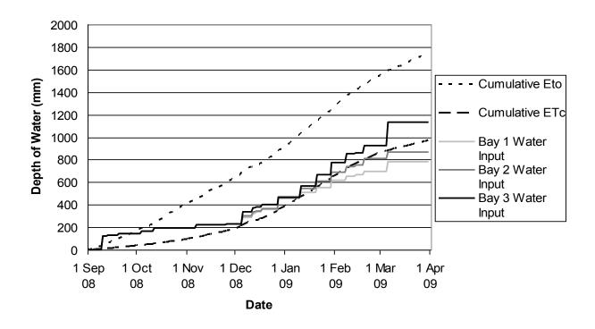
**Figure 4:** ET demand and irrigations applied. Irrigation application data to the 6-Dec-2009 is estimated due to data collection limitations and is assumed to be consistent across all bays.
