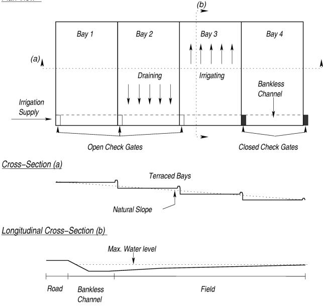
Figure 1: Schematic of bankless channel irrigation system.
