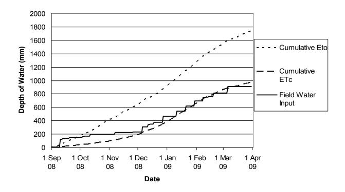
Figure 3: Cumulative ETo, ETc and water inputs for the evaluated field.
