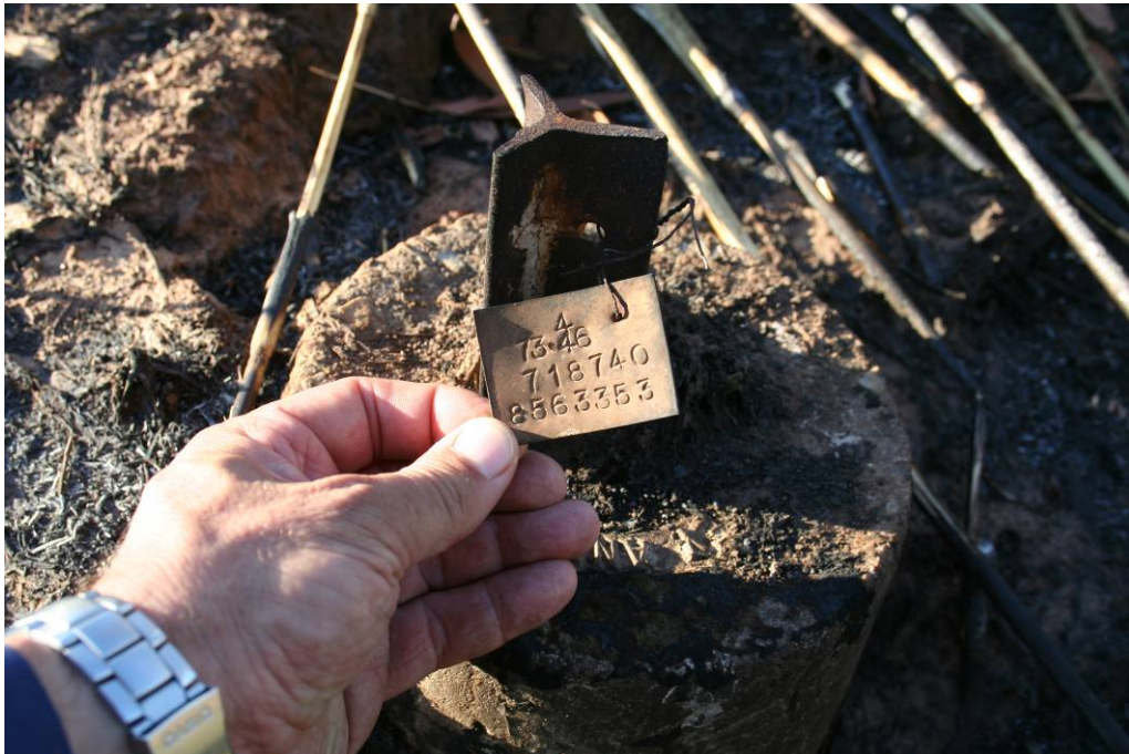
Figure 3.5 Tagged survey monument RL, Easing & Northing
