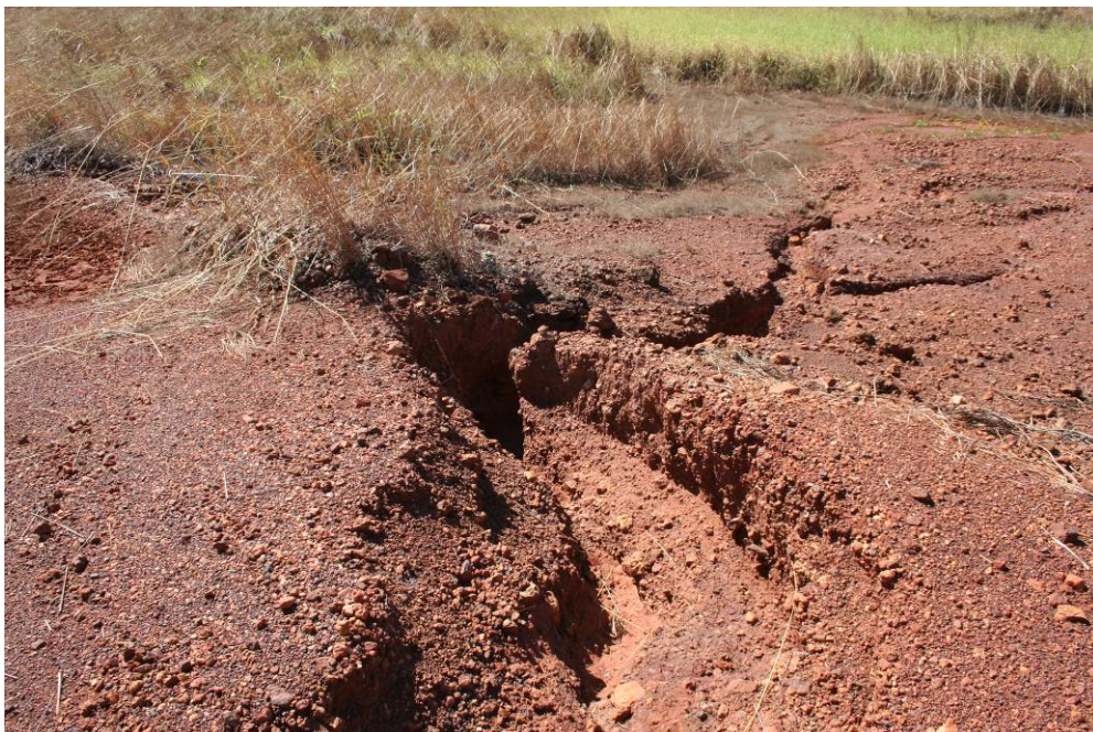
B. 8 Dysons landform, evidence of monsoonal scour at site of maximum settlement, April 2008
