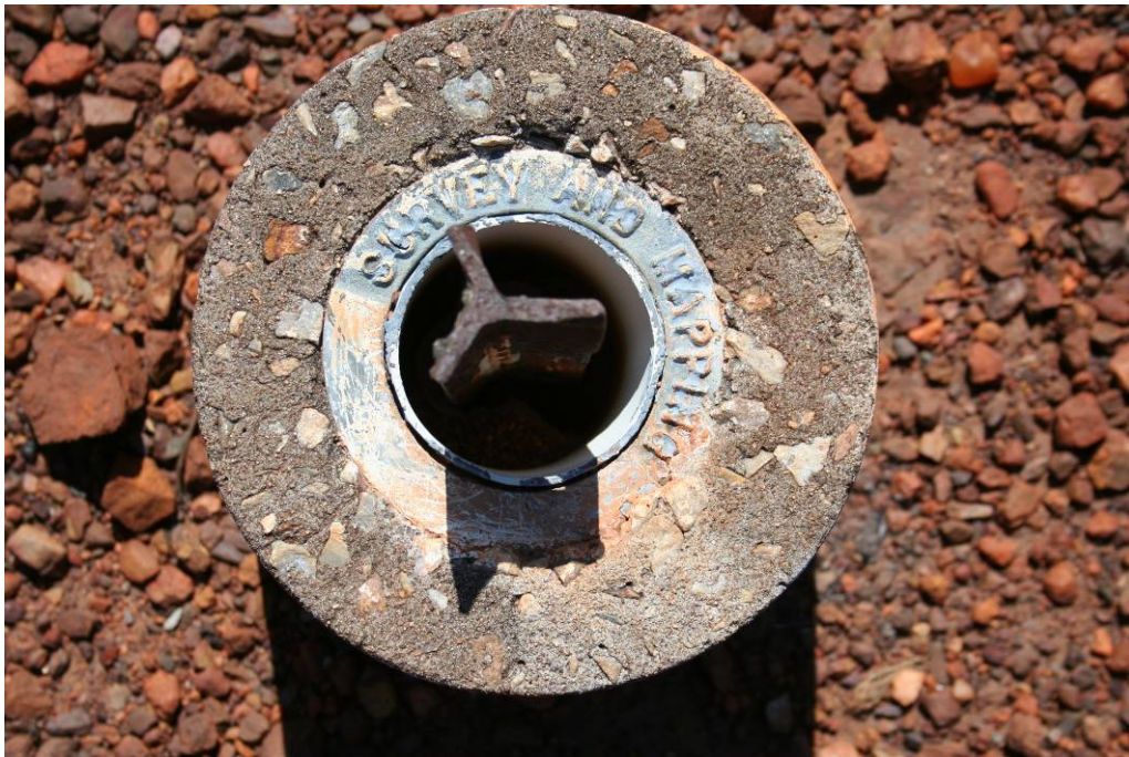
Figure 3.2 Existing survey monument
