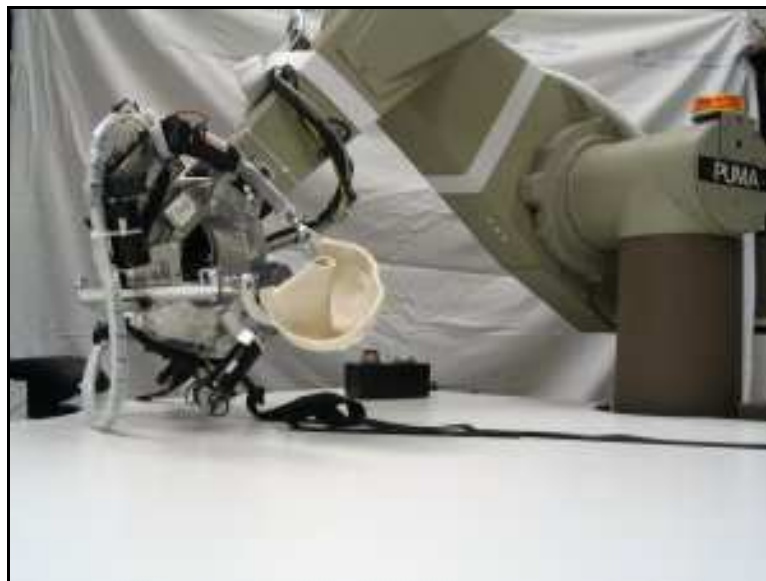
Figure 2-7: modified robot arm (PUMA) (source: Mechatronics and Haptic Interfaces Lab 2008)
