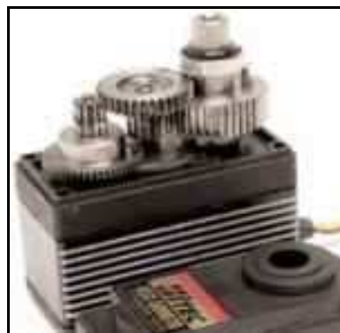
Figure 5-7: servo metal gears
