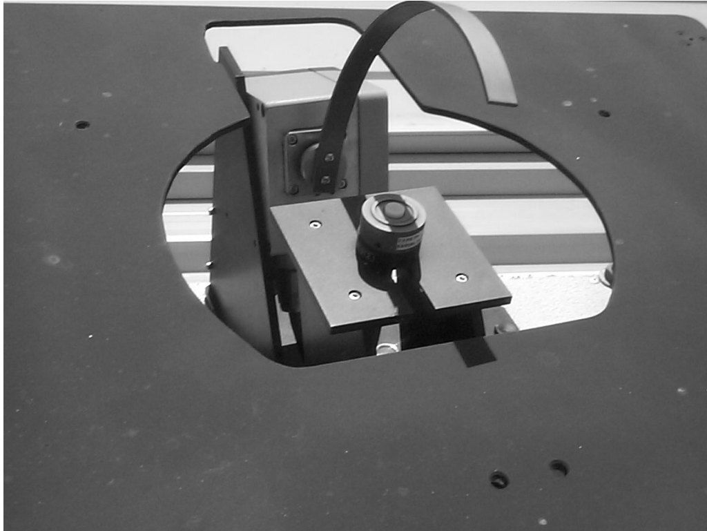
Figure 1 – The configuration of the input optics of the spectroradiometer with the diffuse shadow band in position for the recording of a diffuse UV spectrum.
