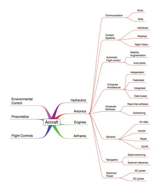
Figure 6-8. Expanded avionics system detail to support development of learning objectives
