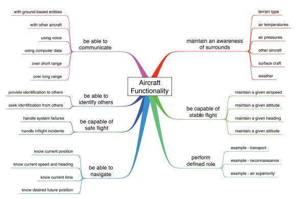
Figure 6-5. Expanded aircraft functionality mind map.
