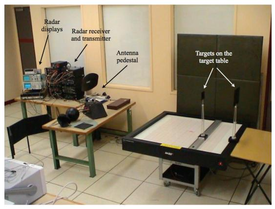
Figure 5-6. The indoor radar trainer consisting of the transmitter, antenna, target, receiver and display.
