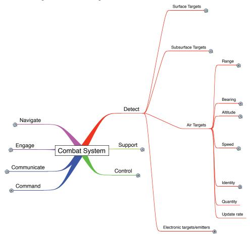
Figure 5-4. Air target information typically provided by radar
