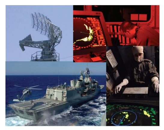
Figure 5-1. The AN/SPS-49 radar system operated by the Royal Australian Navy. Clockwise from top left is the AN/SPS-49 antenna pedestal, a navigation radar display being used by a ship's navigator, a tactical radar display being used by a combat system operator, and an ANZAC Frigate at sea. (Photo sources: author and Department of Defence).
