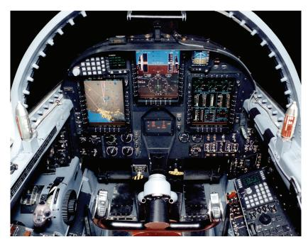
Figure 6-2. Cockpit of the U2 aircraft showing the myriad of displays and controls typical in a modern aircraft (photo courtesy of the United States Air Force).
