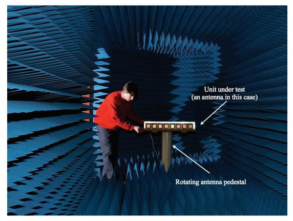
**Figure 5-8.** The anechoic chamber coated in pyramidal radar absorbing material in order to reduce radar reflections off the chamber walls. (Photo courtesy of David Paterson, ETS UNSW@ADFA)
