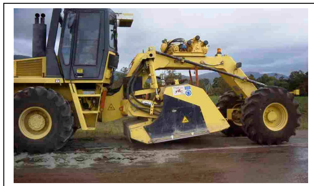
Figure 2-2 - 350 HP Stabiliser Capable of stabilising to a depth of 250 mm.
