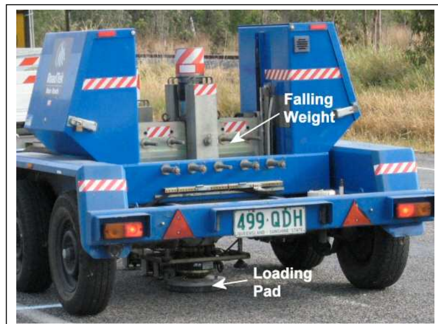
Figure 5-2 - Falling Weight Deflectometer Loading Unit
