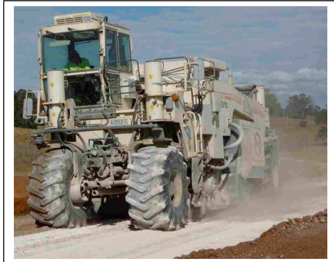
Figure 2-3 - T.R.N. Camden Stabiliser Capable of stabilising to a depth of 500 mm.
