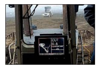
Figure 2.2 Visual Indicator at a Grader (Leica 2007).
