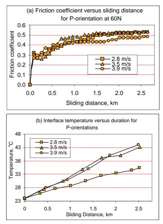
**Fig. 7-** Friction coefficient and interface temperature of CGRP sliding Vs sliding distance showing the effect of sliding velocity P-orientation at 60N applied load
