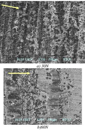
**Fig. 6-SEM** photographs of worn surface for different loads at AP-orientation, 2.8m/s and 2.5 km
