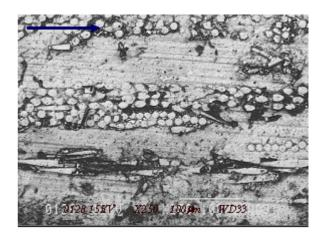
**Fig. 8**-SEM photographs of worn surface of CGRP in P-orientation at 3.9m/s for 2.5km
