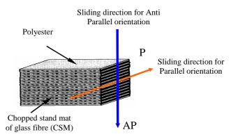
Fig. 1- Schematic illustration of CGRP specimens showing the orientations with respect to sliding direction
