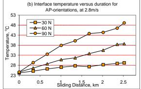
**Fig. 5-** Friction coefficient and interface temperature of CGRP sliding Vs sliding distance showing the effect of applied load in AP-orientation at 2.8 m/s
