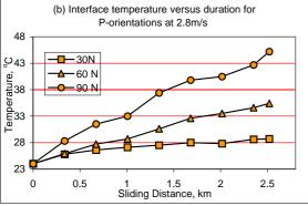
**Fig. 3-** Friction coefficient and interface temperature of CGRP sliding Vs sliding distance showing the effect of applied load in P-orientation at 2.8 m/s
