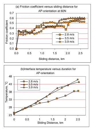
**Fig. 9-** Friction coefficient and interface temperature of CGRP sliding Vs sliding distance showing the effect of sliding velocity AP-orientation at 60N applied load
