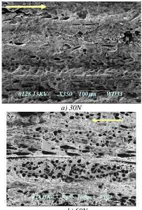
*b)* 60N **Fig. 4-SEM** photographs of worn surface for different loads at P-orientation, 2.8m/s and 2 km.
