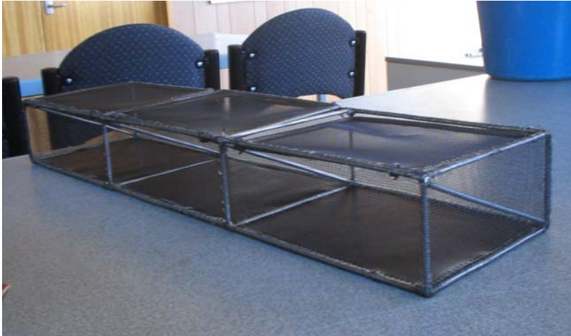
Figure 3.1 Constructed weir minus the porous media
