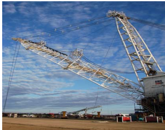
Fig. 6.3 Bucyrus Tubular design boom
