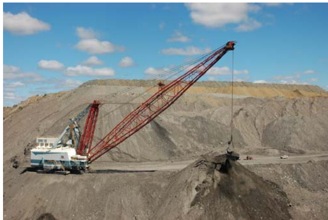
Fig. 2.1 - Marion 8050 Boom length 84 to 108m-Bucket capacity 43 to 71 m 3 -Max operating weight 3,629tonne
