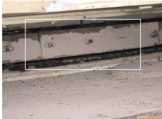
Fig. 6.4 Roller Circle connecting revolving frame to tub
