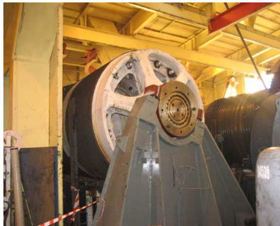
Fig. 6.5 Modified winch drum bearing Larger diameter and width bearing installed
