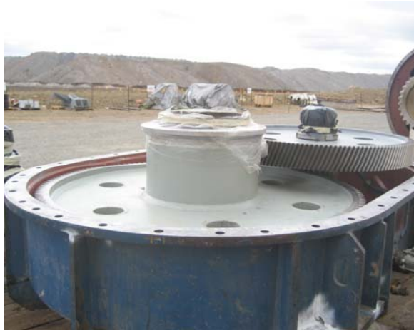
Fig. 6.8 Helical cut gears in swing gear case
