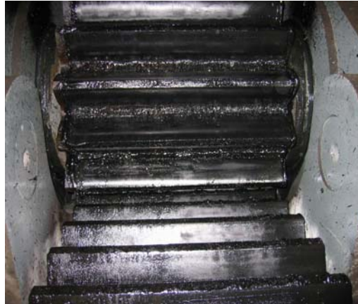
Fig. 6.7 Propel spur gears. Lubricant is high pressure grease
