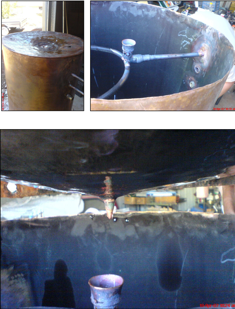
Figure 3.28: Condenser System (Note the tapered in lid)
