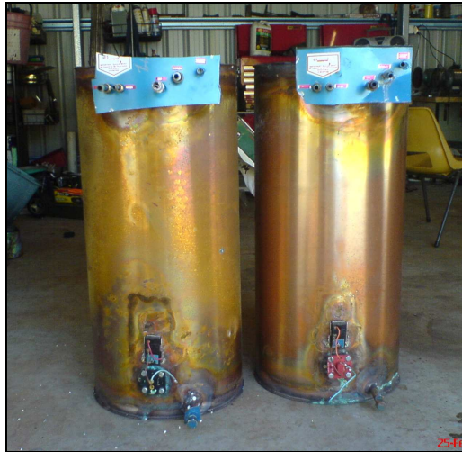
Figure 3.26: Copper hot water system tanks
