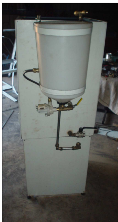
Figure 3.30: Recirculation System + Alcohol and Acid Mixing System
