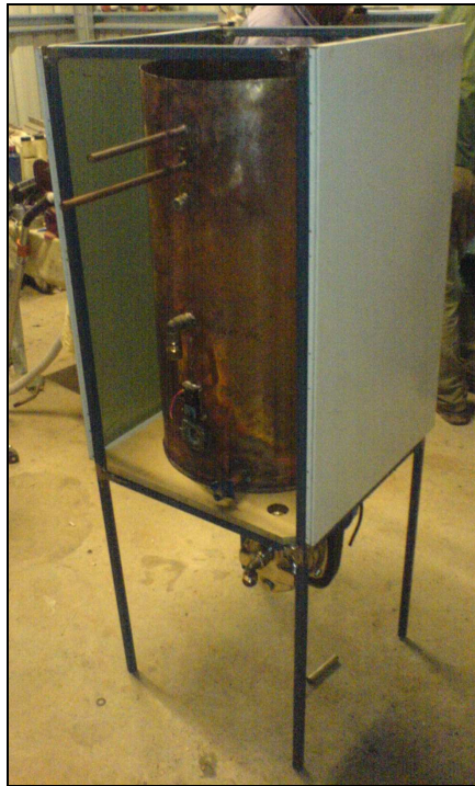
Figure 3.29: Reactor Vessel and Recirculation pump fixed and located.
