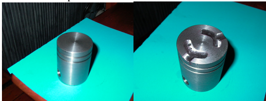
Figure 9. Piston modification after initial tests indicated that flame propagation was a problem
