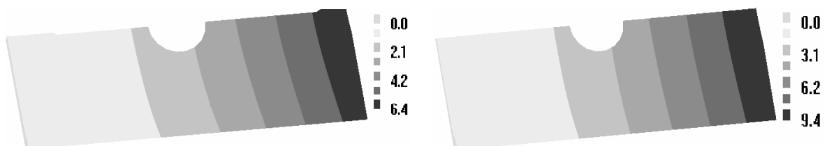
(d) Final optimized plate of 4 mm thick, with three sets of ribs of 3 mm thick, after four rounds of optimization procedure.
