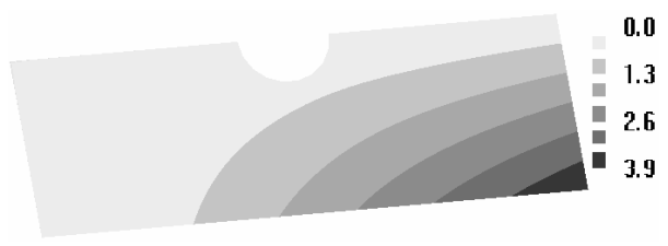
(d) Final optimized plate of 4 mm thick, with three sets of ribs of 3 mm thick, after three rounds of optimization procedure.
