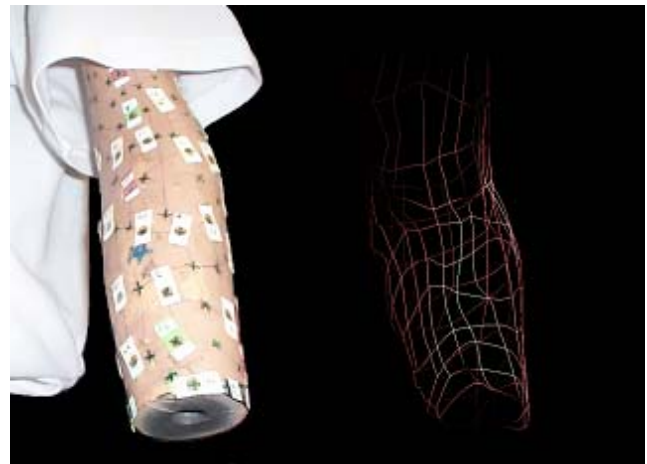
Figure 1. Photographed manikin arm dosimeter sites (left) and three dimensional model exposure contours (right). ER was measured for the arm in a vertical position (alongside the manikin as photographed). The ER depicted here ranges from 0 to 51% (dark to light) of the measured horizontal plane UV_{ery} exposure.
