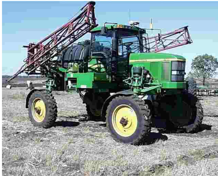
Figure 1: GPS and Radio Antennae on Spray Rig
