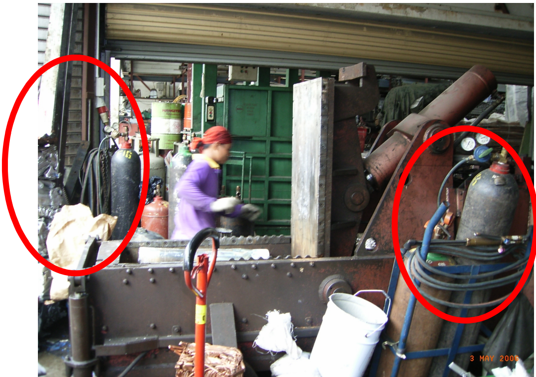
Figure 4.3 Dangerous Placement of Machine
