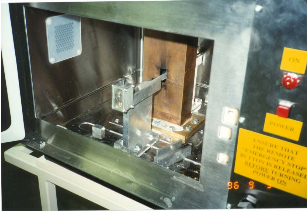
Figure 3: Slotted Rectangular Waveguide Used for Joining LDPE/CF (33%) with Araldite Using Fixed Frequency Equipment
