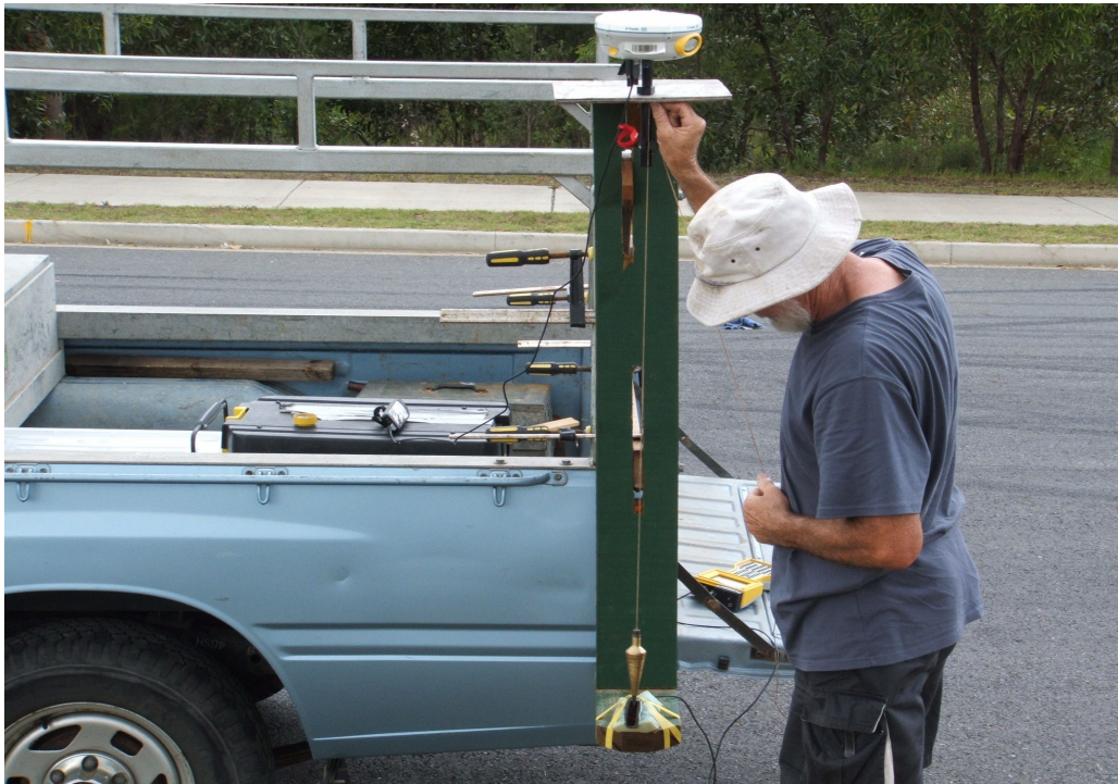
Figure 3.2 – Using a Plumb-bob to check the Antenna / Barcode Reader Alignment. (Author)
