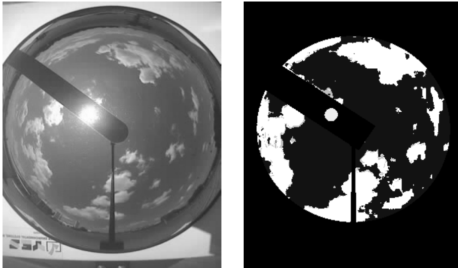
Figure 4.11. Examples of an unprocessed and processed total sky image for quantifying cloud cover (31% cloud cover in this case).
