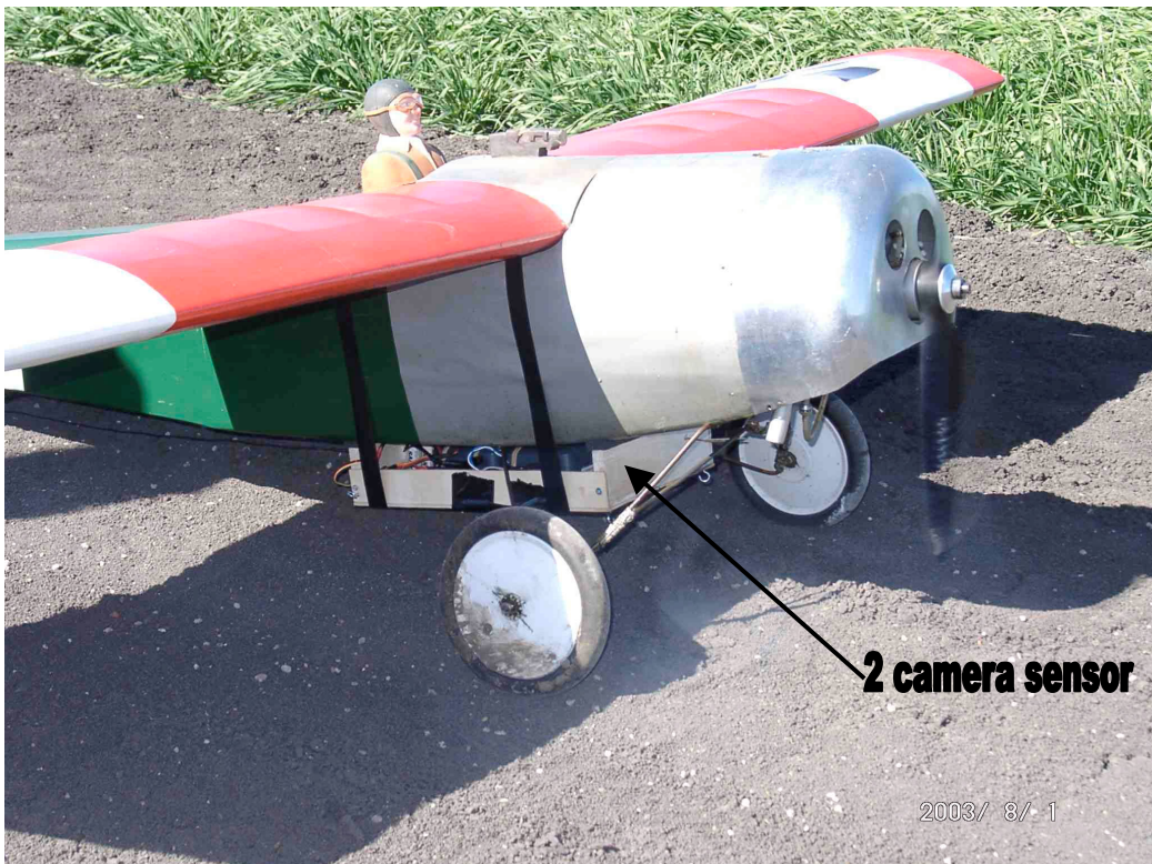
Figure 7 The current platform with the sensor taped beneath the fuselage
