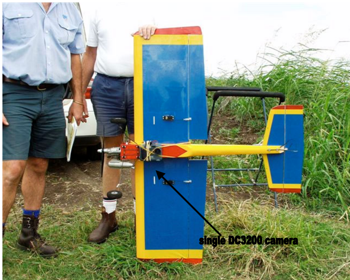
Figure 1 The image acquisition system incorporating the digital camera sensor and the remote control aircraft platform
