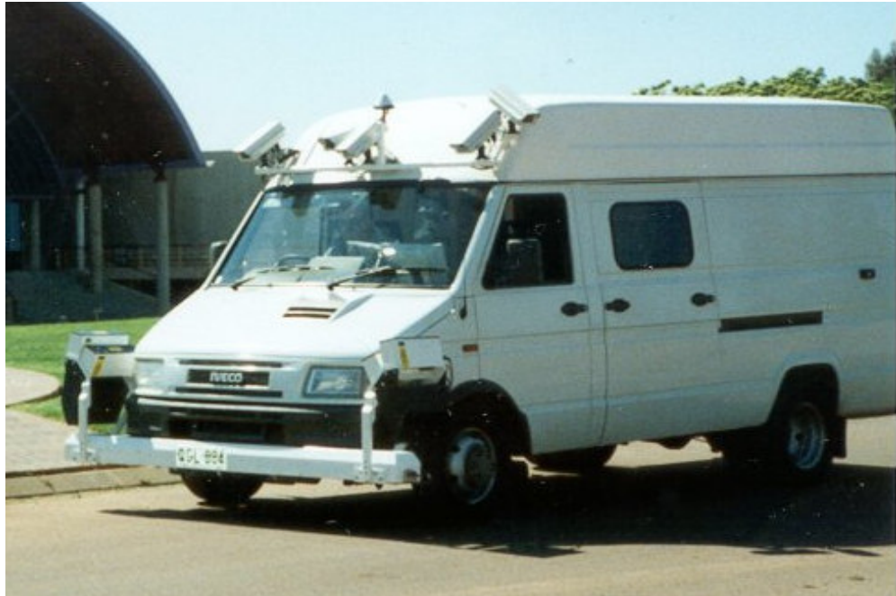
Figure 4.5 Network Survey Vehicle (Source: Courtesy Ed Baran)
