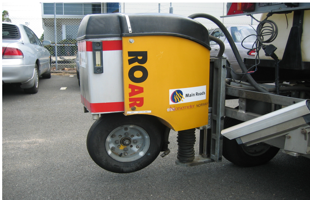
Figure 4.1: Norsemeter ROAR Skid Tester (Source: Courtesy E. Baran)
