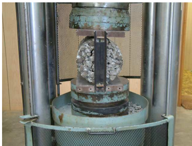
Figure 7.8 – The compression machine is set up for an indirect tensile test
