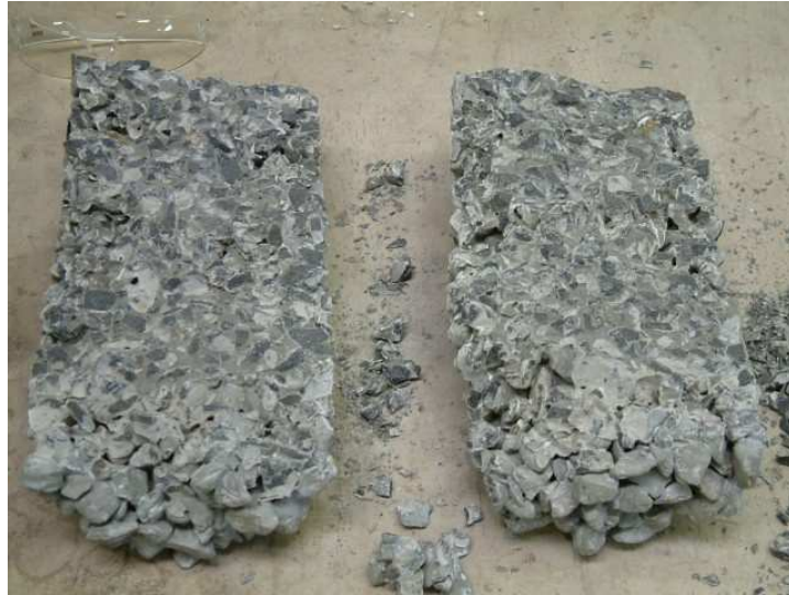
Figure 7.10 – The failure of the no-fines concrete after an Indirect Tensile Test
