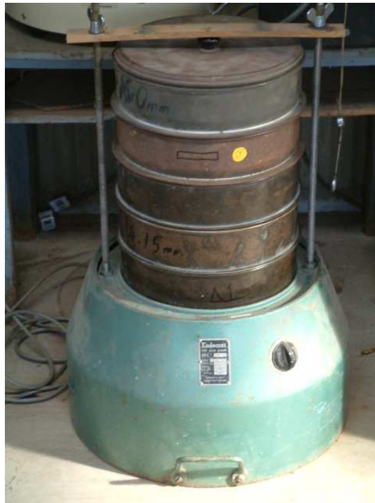
Figure 5.1 – The shaking device and stack of sieves used to conduct the sieve analysis
