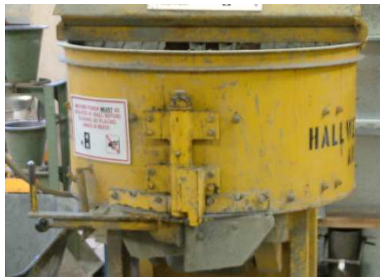
Figure 6.1 – The Hallweld Bennett Pan Mixer used for the no-fines concrete mixes
