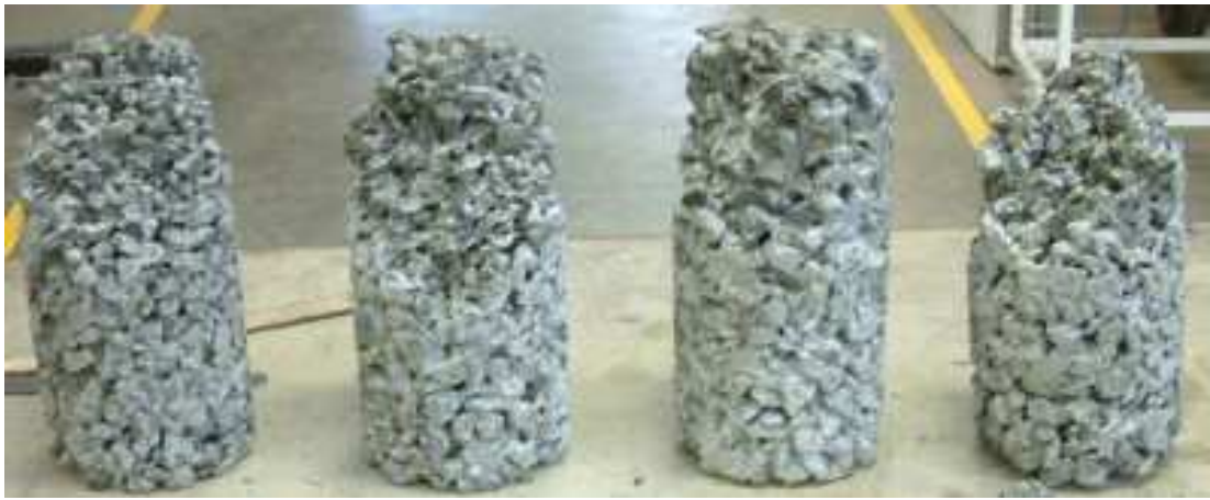
Figure 4.4 – Shows the failure of the four mixes on the large cylinders
