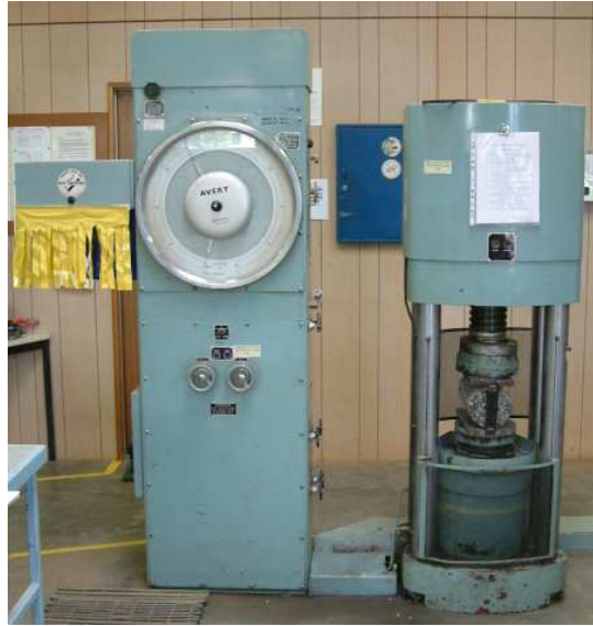
Figure 7.2 – Avery machine used to conduct the concrete testing
