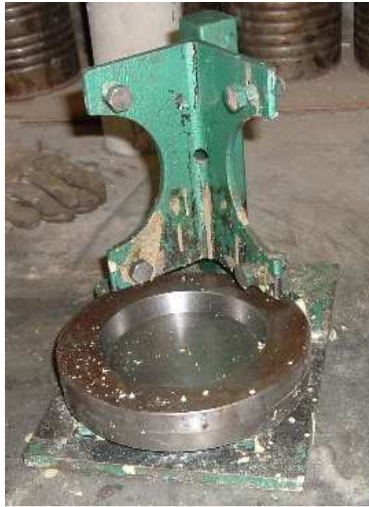
Figure 7.1 – The capping mould used for sulphur capping
