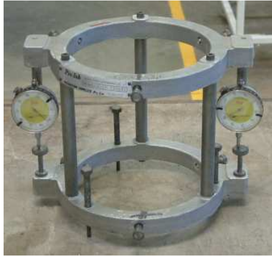
Figure 7.16 – Typical compressometer used to measure the longitudinal strain
