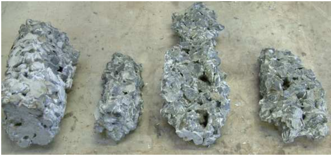
Figure 4.3 – Shows the failure of Mixes 3 and 4
