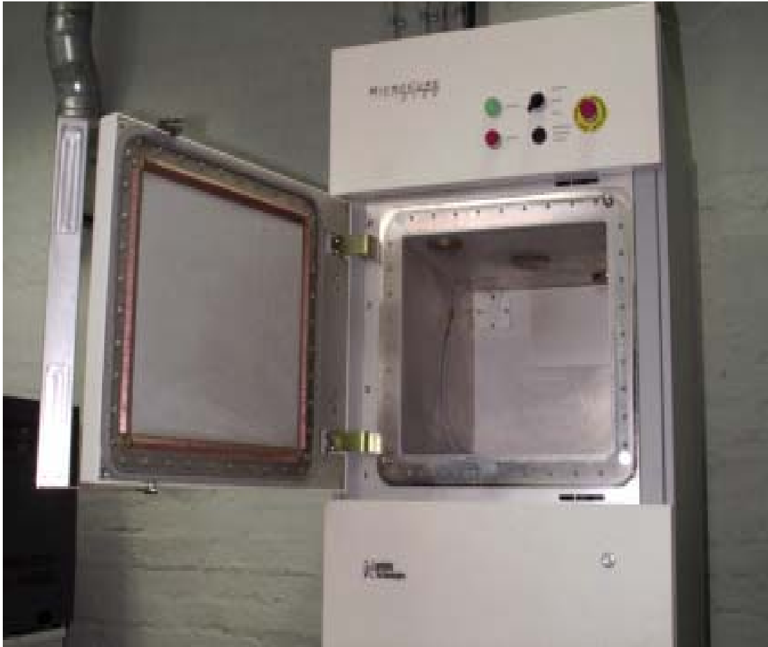
Figure 1: Cavity of Microcure 2100 Model 250 with a Frequency Range of 2 - 7 GHz and a Maximum Power of 250 W
