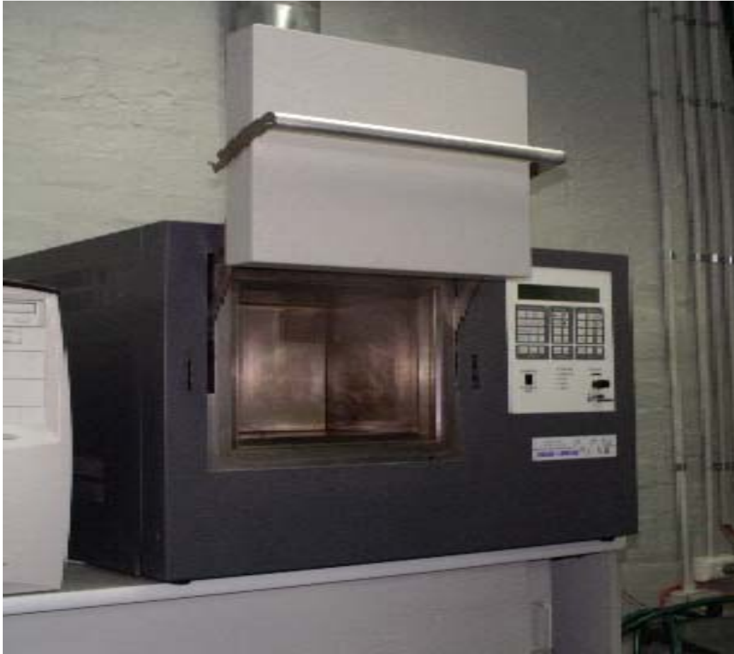
Figure 2: Cavity of VW 1500 Model with a Frequency range of 6-18 GHz and a Maximum Power of 125 W
