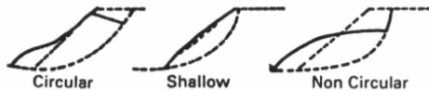
Figure 2.2 Rotational slides ( Slips & Slumps) (Raj, 1995)
