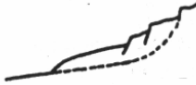
Figure 2.8 Slump earth flow (Raj, 1995)
