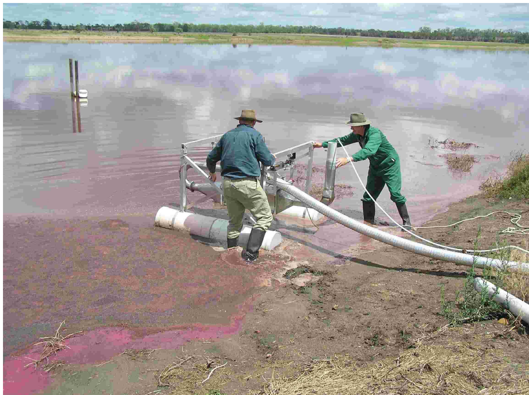
Figure 3.1: Launching the Wind Tunnel onto the Pond Surface
