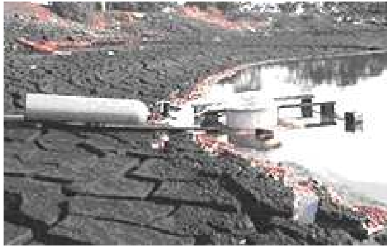
Figure 2.1: Flux Hood in use on an effluent pond (taken from http://www.odour.unsw.edu.au/flux-hood-sampling.html )
