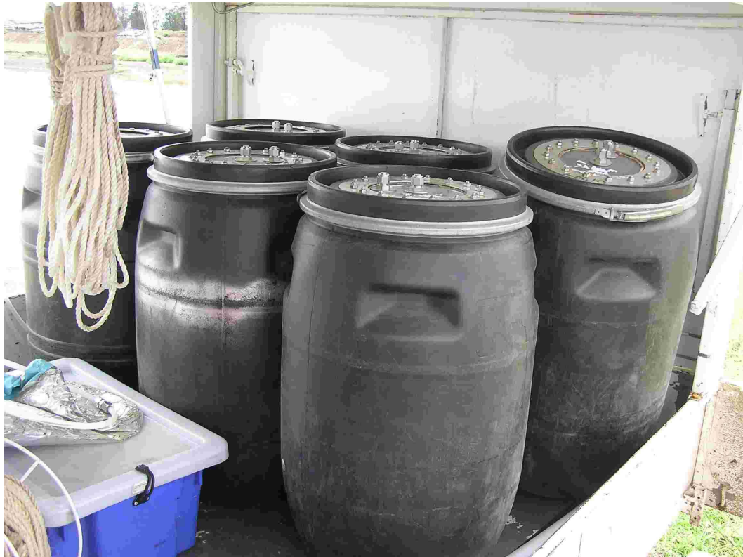
Figure 3.5: Odorous Air Sample Collection Drums
