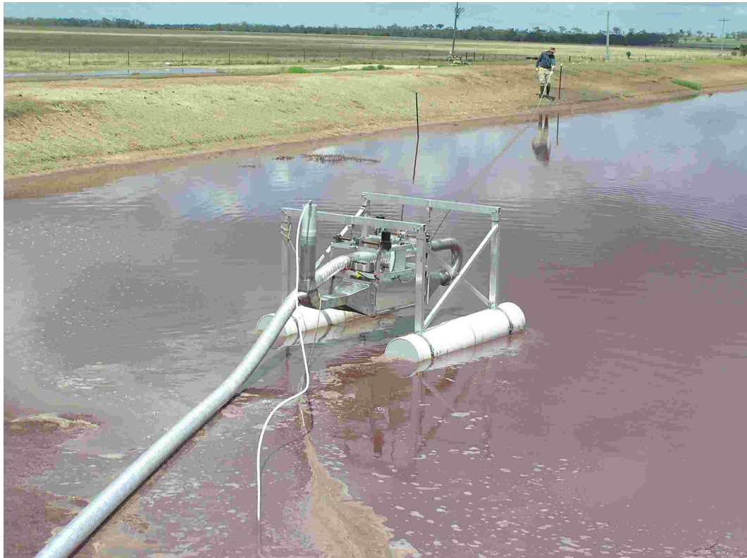
Figure 3.3: Wind Tunnel, Ready to be lowered into Sampling Position
