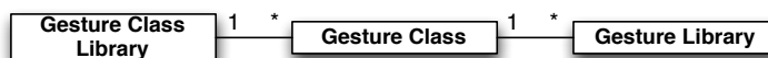
Figure 5.4: UML object diagram showing the relationship between the gesture class library, gesture classes and gesture traces.
