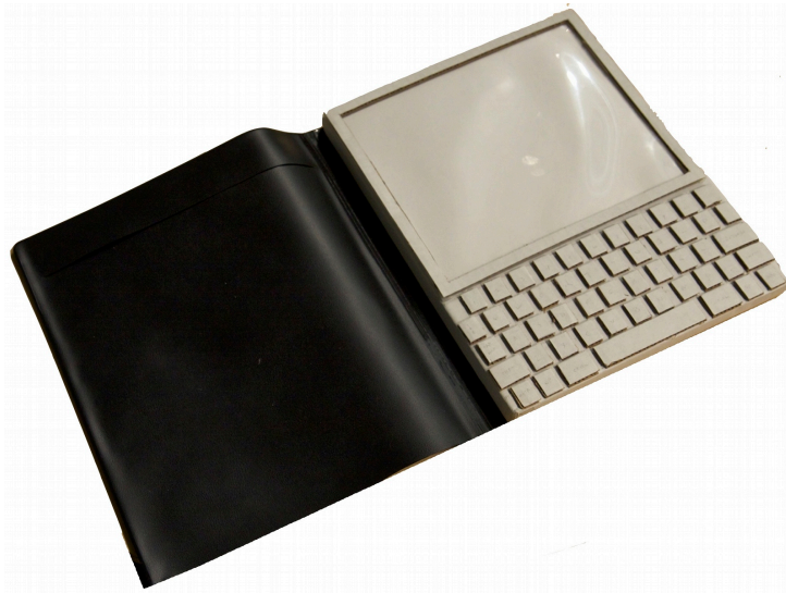
Figure 1.1: Alan Kay's original DynaBook paper prototype. Adapted from original image by Flickr User Marcin Wichary ©(P).
