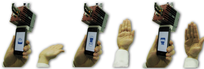
Figure 4.8: Using the pose of the flat hand behind the device to freely rotate a 3D object. A depth camera is used to determine the hand posture. (Kratz et al., 2012a).
