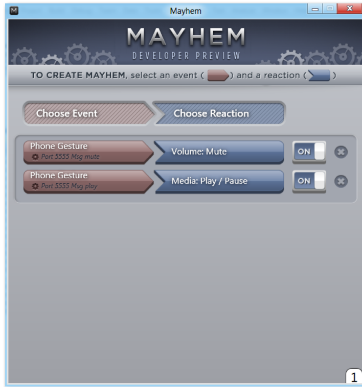
Figure 6.6: Mayhem configuration that is used to control the media player via phone gestures.
