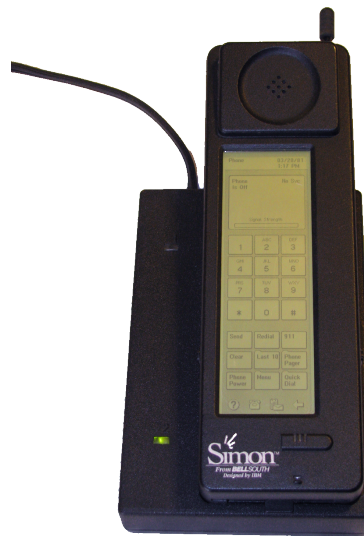
Figure 1.3: The IBM Simon in its charging cradle. The large touch-screen with on-screen keyboard for dialing is visible.
